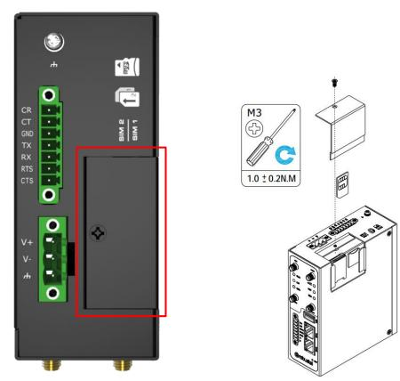
Insert or remove the SIM/Micro SD card as shown in the following steps.
