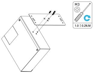
Use 3 pcs of M3\*4 flat head Phillips screws to fix the wall mounting kit to the router, and then use 2 pcs of M3 drywall screws to mount the router associated with the wall mounting kit on the wall. **Note:** Recommended torque for mounting is 1.0 N.m, and the maximum allowed is 1.2 N.m.
