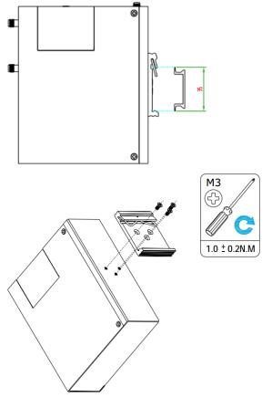
Use 3 pcs of M3\*6 flat head Phillips screws to fix the DIN rail to the router, and then hang the DIN rail on the mounting bracket. It is necessary to choose a standard bracket.
