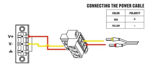
R3000 Router supports reverse polarity protection, but always refers to the figure above to connect the power adapter correctly. There are two cables associated with the power adapter. Following to the color of the head, connect the cable marked red to the positive pole through a terminal block, and connect the yellow one to the negative in the same way. The last step is to plug the power adapter into your socket. **Note:** The range of power voltage is 9 to 60V DC.
